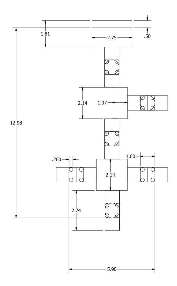
Sketch drawing of base plate for small tube manifold on M2 and M1. 9/8/2017 version 1
